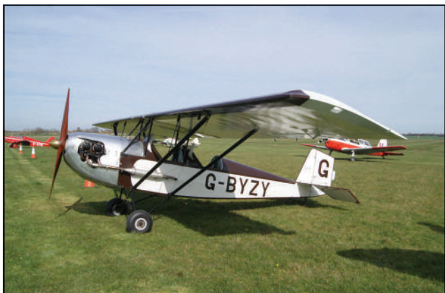
Each of these aeroplanes having different power plants giving entirely different contours to the shape of the front of the fuselage.
